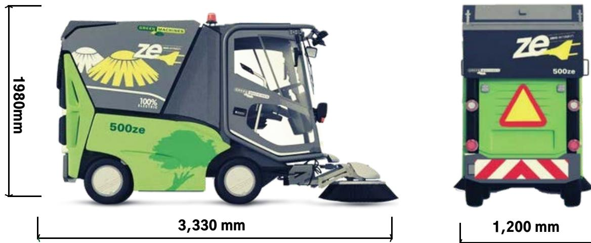
All measurements in millimetres
